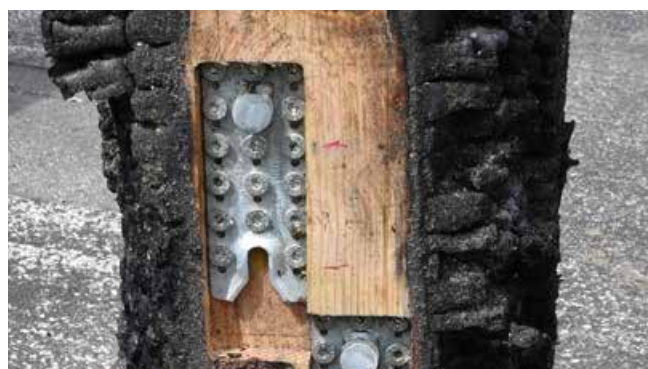
RICON® S connector after fire testing for 90 minutes. The wood is charred all around. During the fire test the connector consistently held the applied vertical load.
