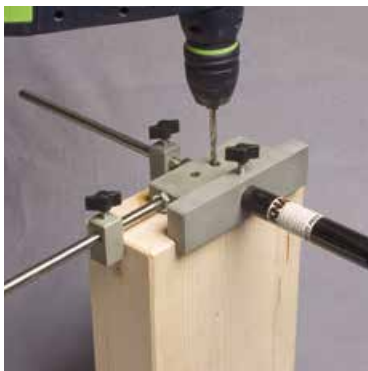
4) Pre-drilling secondary beam
