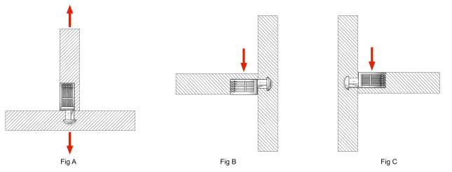
**PEANUT**® 1 Tensile/shear strength (based on 2 components)
