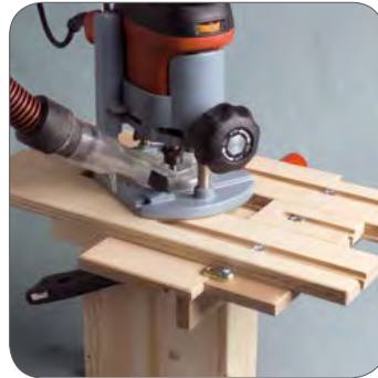
1) Routing with routing-jig and routing machine.
