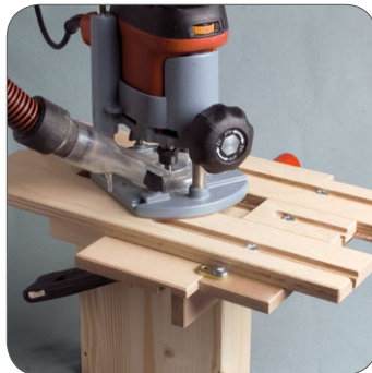
1) Routing with routing-jig and routing machine.
