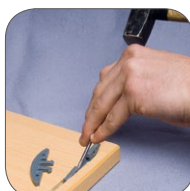
3) Knock in with the insert tool
