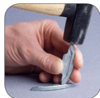
2) Bending locking clips
