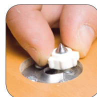
3) Transfer with the center punch
