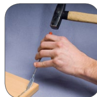
4) Knock in with the insert tool
