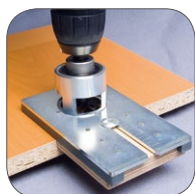
1) Drilling with jig
