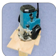
1) Route with routing-jig
