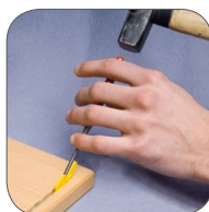
3) Knock in with the insert tool
