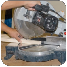
1) Cut to size glass bar and FIXclip-Profile
