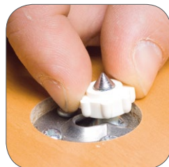
3) Transfer with the center punch
