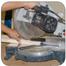
1) Cut to size glass bar and FIXclip-Profile
