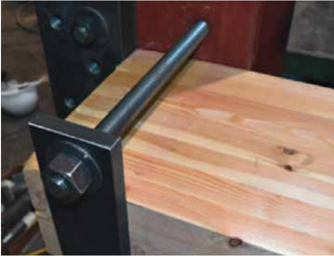
Figure 6: Threaded rod tie to reaction frame at post member
