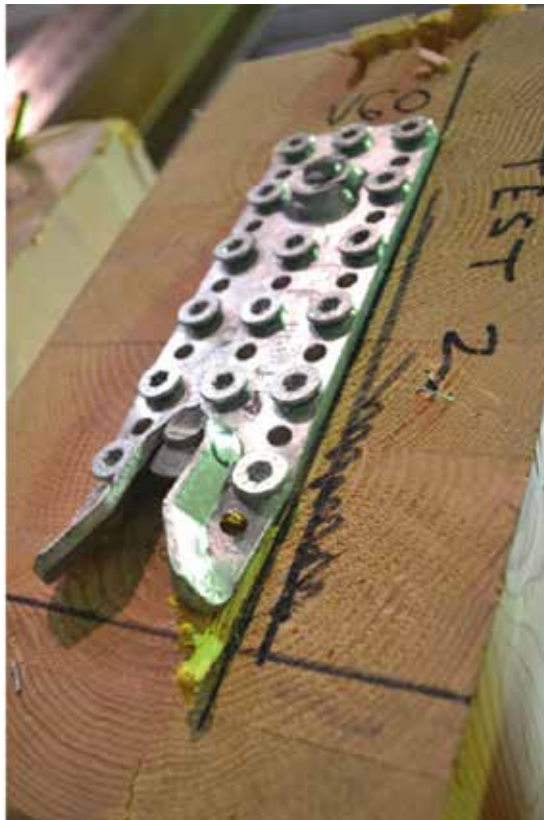
Figure 15: Collar bolt failure in beam member RICON® SVS 200x60
