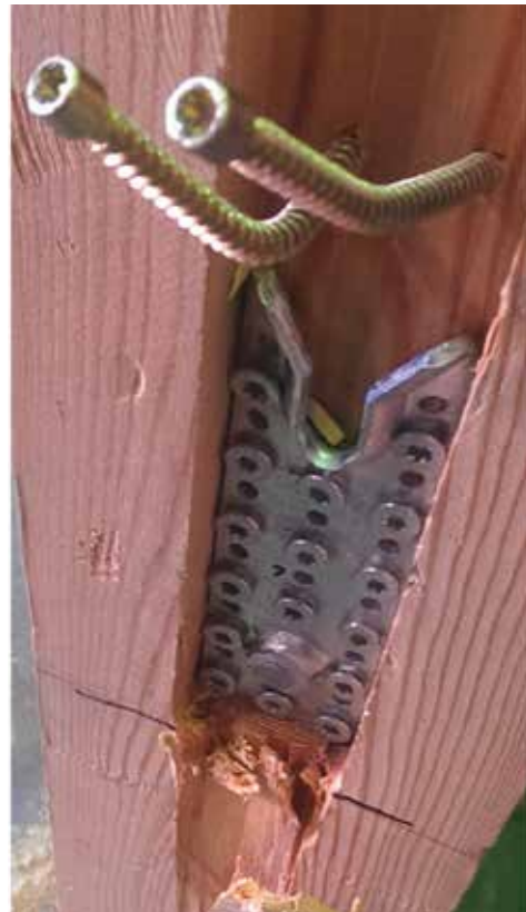
Figure 16: V-notch yielding in post member and yielding toe screws
