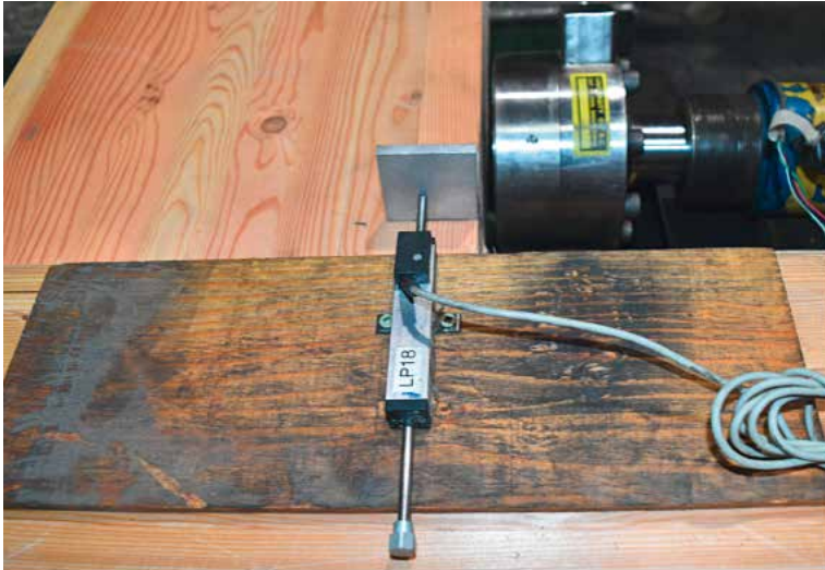
Figure 3: Displacement recording (#1) at interface of beam and column and constant design shear load application actuator (#2)
