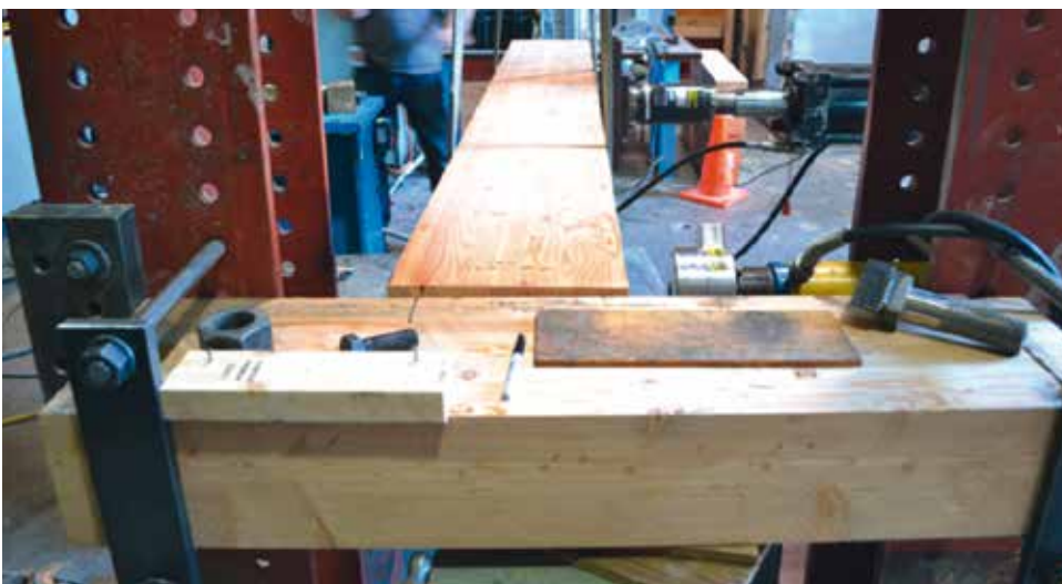
Figure 8: Reaction frame with specimen
