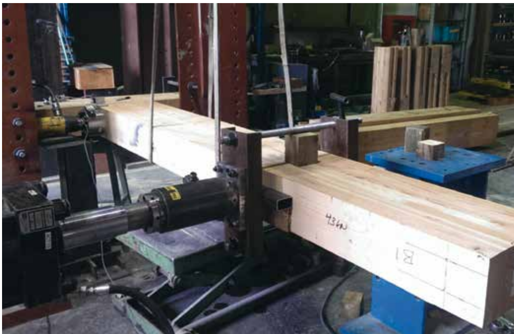
Figure 1: General Test setup and typical RICON® S VS connector
