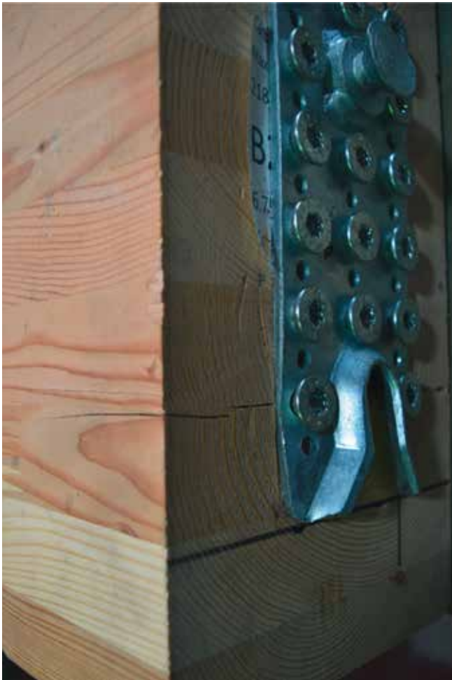
Figure 19: Collar bolt yielding at RICON® S VS 200x80 connector
