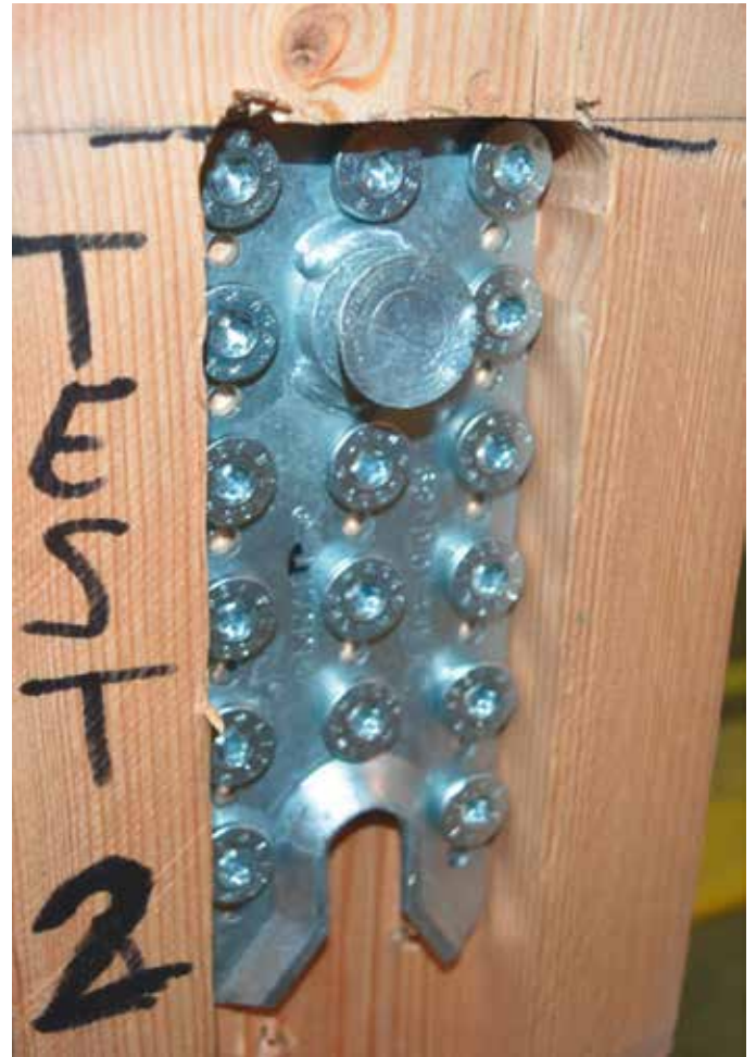
Figure 20: Flange yielding at RICON® S VS 200x80
