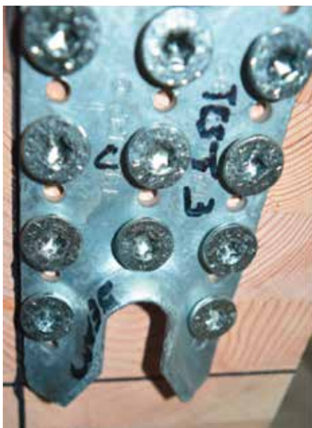
Figure 21: Elastic deformation at V-Notch
