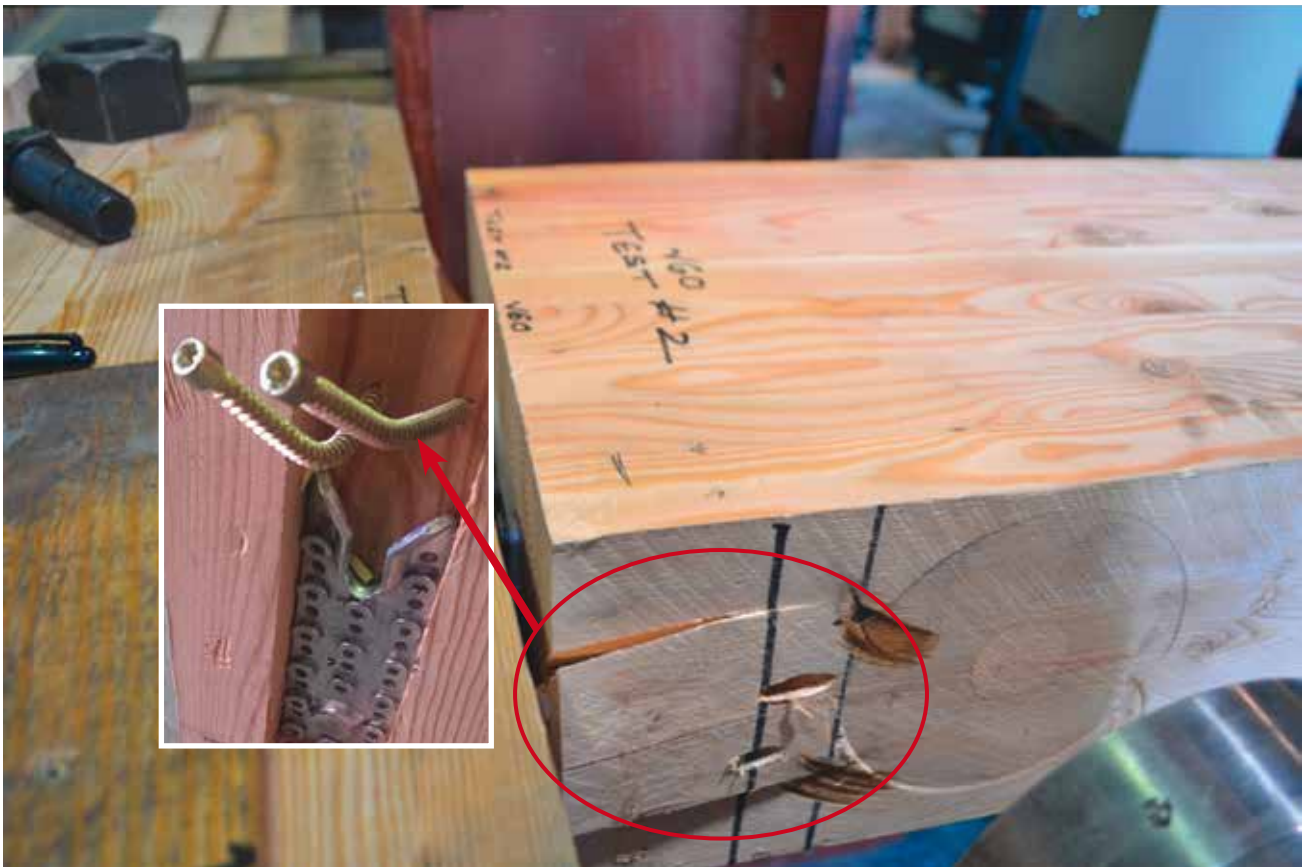
Figure 18: Splitting of beam edge after failure occurred in collar bolt. Uplift toe screws yield
