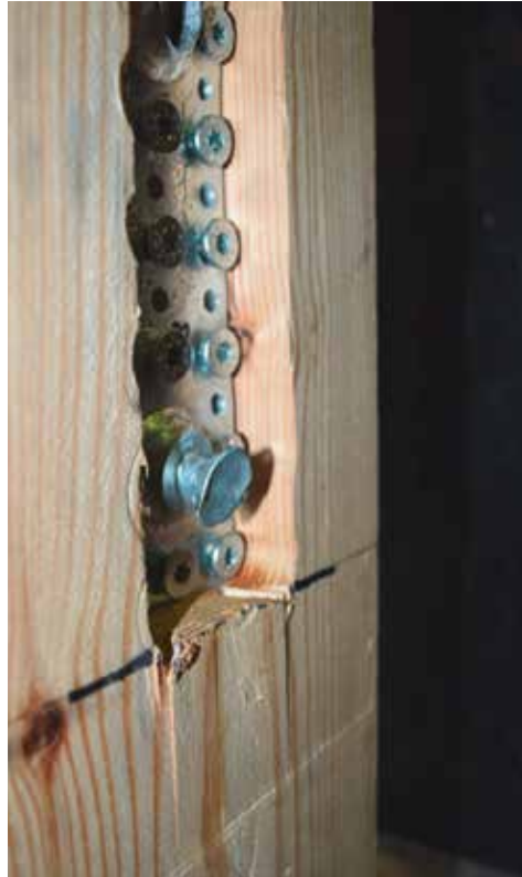
Figure 14: Collar bolt yielding post member
