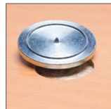
Transfer with the centre punch
